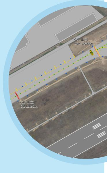
The position of the new holding point is by 247m closer to the runway, allowing aircraft to line up and take-off in a more expeditious way in low visibility conditions.
